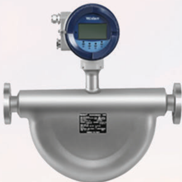
CORIOLIS FM, UP TO 200 BAR, 260,000 KG/H HART, MODBUS FF AND PROFIBUS PROTOCOLS
